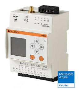
RTUEVO1T (1.ETRSEQ.0051) is a datalogger to acquire data from 1.ETRSEQ.0012, which, through the mesh network, collect information from devices that use M-Bus wired and wireless protocol such as meters, heat cost allocators, probes. Manages up to 3000 meters (2500 wireless + 500 wired devices) providing storage of daily readings for 10 years. The web interface allows accessing data, reports generating, setup of the M-Bus and MESH networks.
